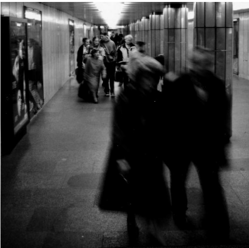
Figure 11. This photograph of a pedestrian tunnel connecting two subways in Budapest at Deák tér illustrates that a series of columns acts like a wall and stabilizes lanes (by preventing the lane width from exceeding half of the total width of the walkway).
